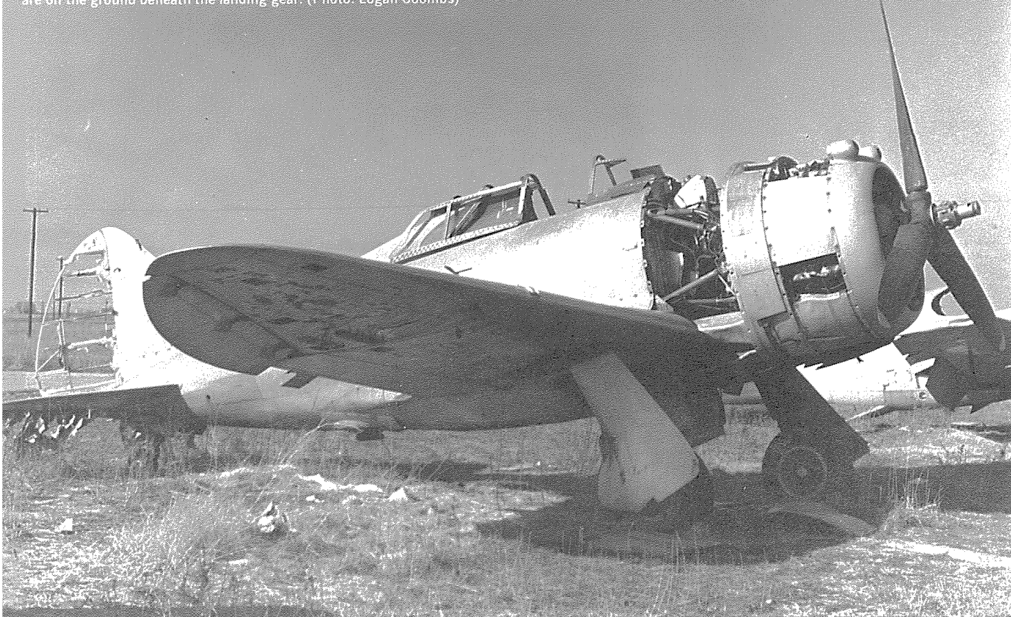
Republic P-43A sitting in the grass deteriorating due to neglect in the fall of 1952. Note that several pieces have been removed from the fuselage and are on the ground beneath the landing gear. (Photo: Logan Coombs)
