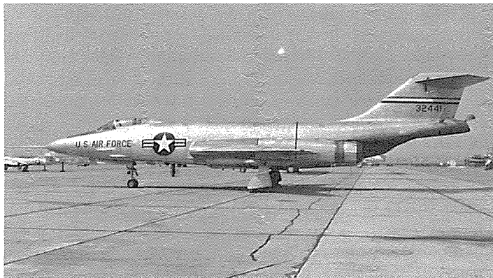
A late pre-production model F-101 shows the noticeable difference between the record setting aircraft and the standard J57-P-13 engine configuration. (Photo: Peter Bowers via Jim Sullivan)
