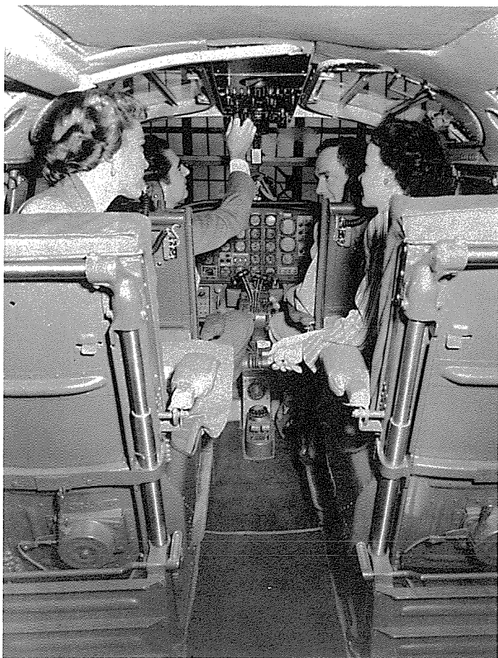
Bearing no resemblance to standard B-25s, the widened cockpit area of N5126N featured comfortable seating for four. Note the Convair 240 instrument panel.
