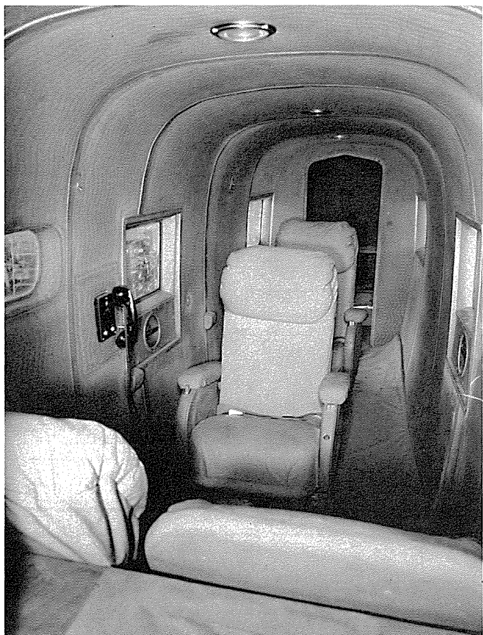
Neither 'posh' nor spacious by modern standards, old No. 1 provided comfort with lots of convenience. The quilted upholstery, known as 'skyfelt', was commonly used for insulating heating and ventilating ducts.
