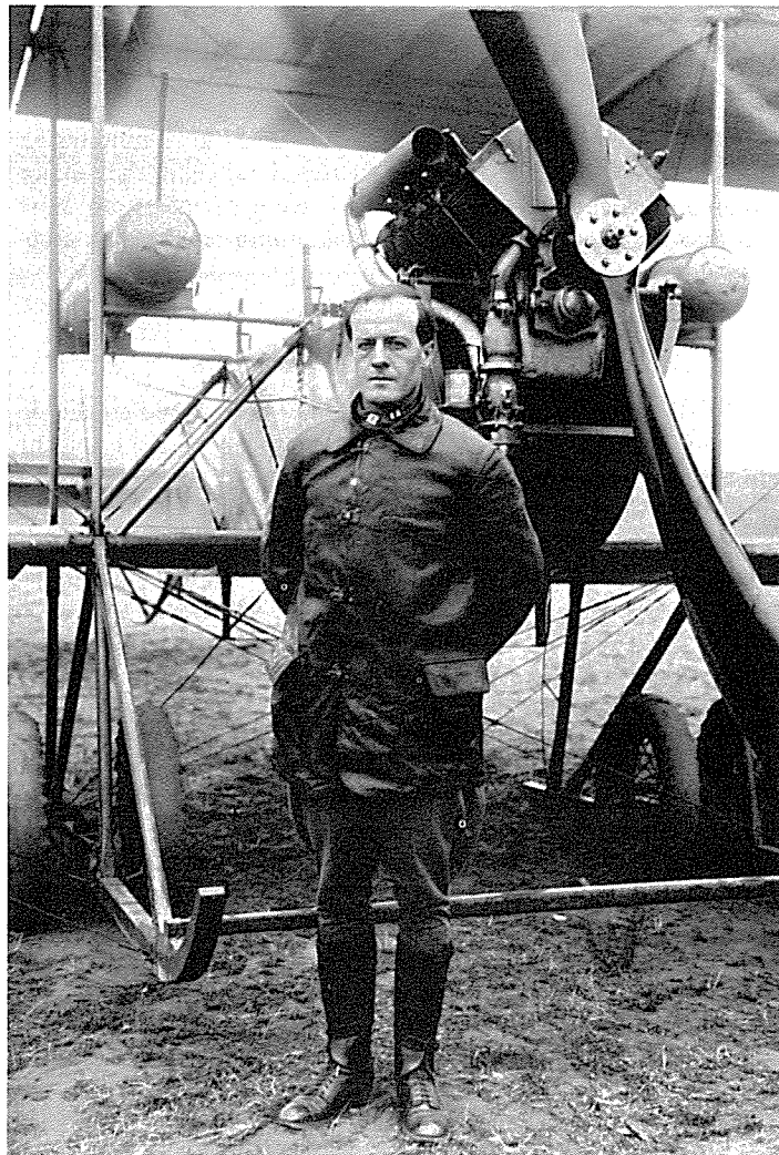
Captain Benjamin D. Foulois with a Burgess H in July 1914. Installation of the 70-h.p. Renault is essentially identical to that in Number 9 of 1912.
