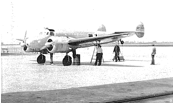
AE’s Electra just outside the Mantz hangar at Burbank. Apparently this was some sort of fuel check since the compass rose at Burbank was located in another area; note fuel under a/c. It is interesting to note the spinners. As far as is known this was the first this modification has been shown. (Dusty Carter collection)
