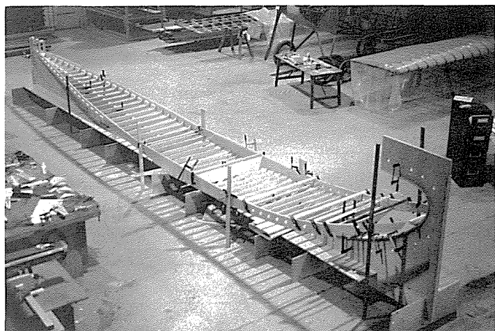
Curtiss HS-2L hull under construction at Ottawa, Canada, November, 1975. This will be assembled with wings and tail surfaces from C-652. Fokker D-VII under restoration in background. (Photo by K.M. Molson)
