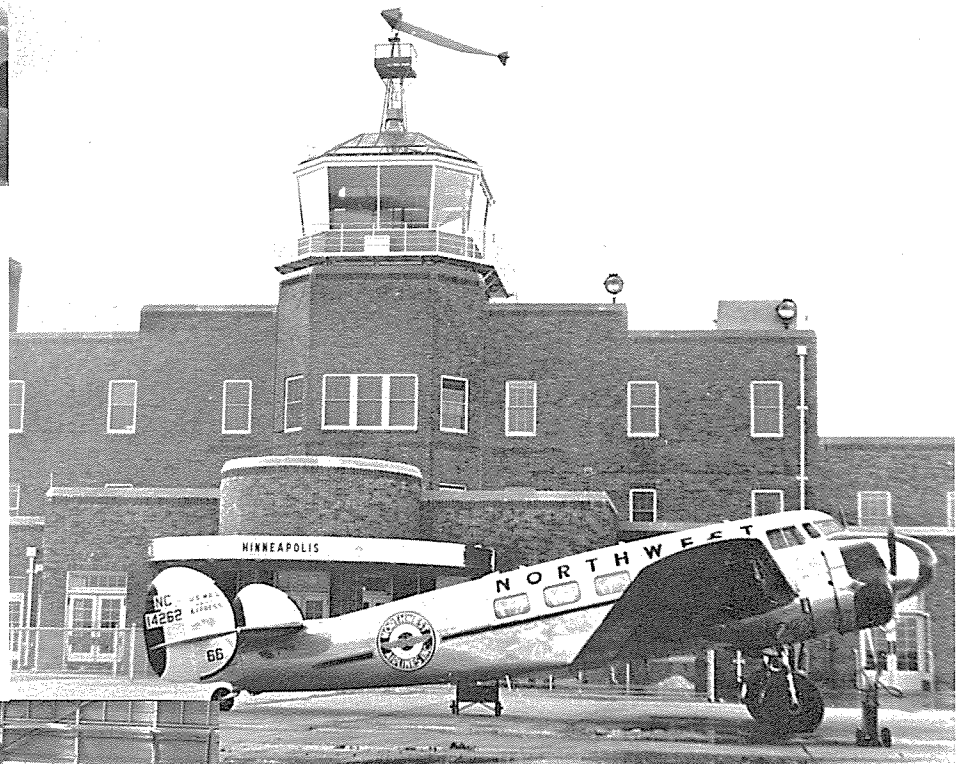
(Below) Lockheed 14-H2 NC18994 was last of 11 Super Electras delivered to Northwest, and bore the c/n 1439A. It replaced NC17394 (c/n 1439) which crashed prior to delivery. Balance panels are evident on the rudder. (G. Williams via James Borden)
