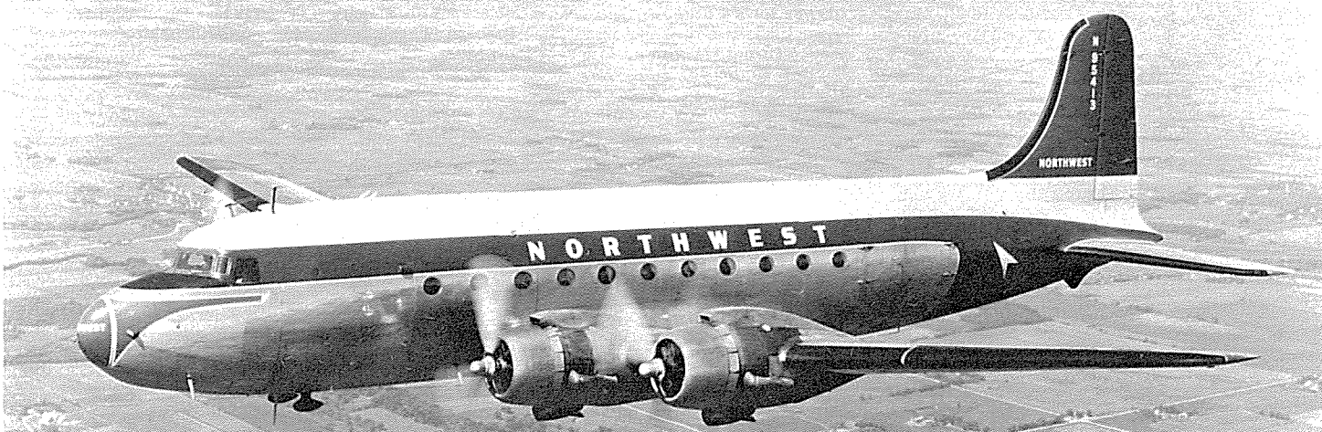
N95413, Northwest's third of over 40 DC-4s, was a modified C-54 purchased shortly after WW II. Passenger capacities varied from 32 to 66, but most were configured for 50 or 62. (Northwest Airlines)
