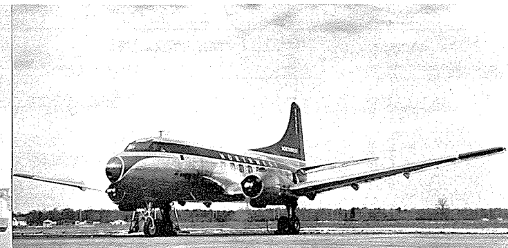
(Below) Greatly increased dihedral and modified tail of Martin 202 is illustrated by NC93047 during run-up test. Only 25 of order for 40 were delivered. (Northwest Airlines)
