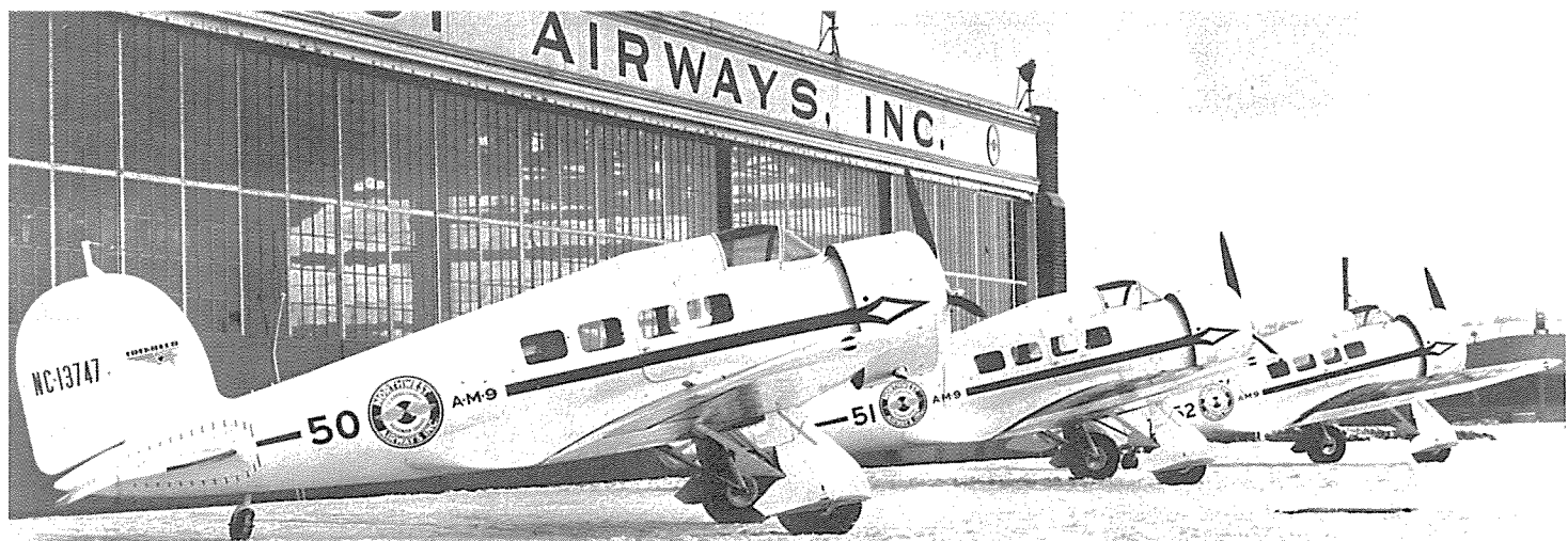
(Above) All 3 Lockheed Orions pose at St. Paul on January 8, 1934. Fleet number 50 and 51 have 3-blade props, while 52 carries a 2-blade. Other photos show varying combinations. The wooden Orions weighed up to 5800 pounds at takeoff, and cost $19,500 each. (George Johnsen via James Borden)
