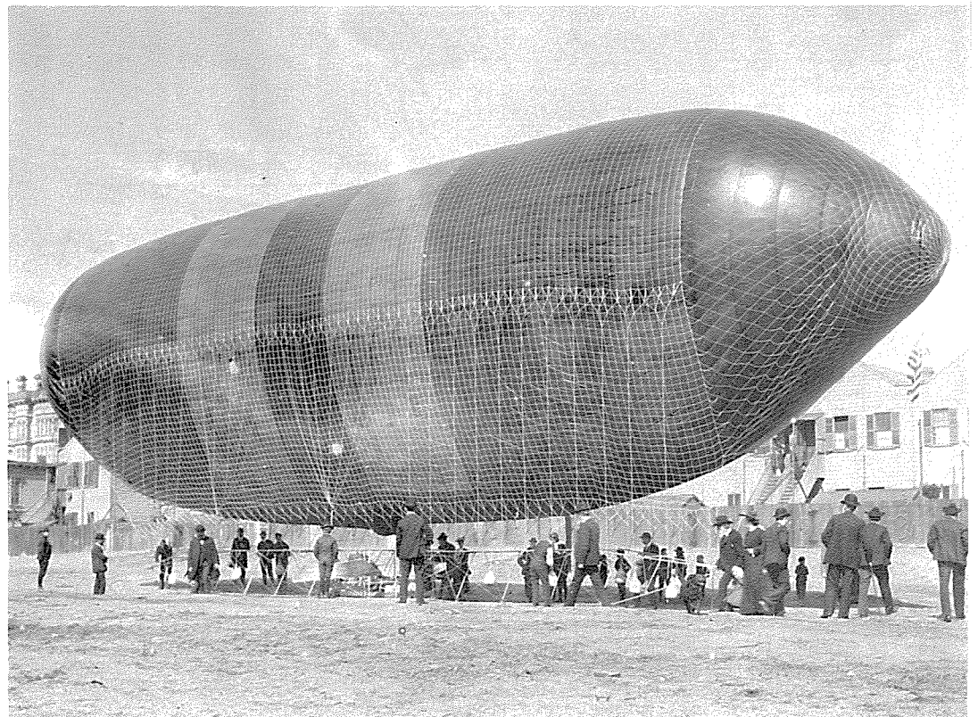
The photos on these pages were probably taken of the California Eagle on August 10, 1903, when the airship had a full-length keel girder, no rudder, and with the propeller shafts mounted low in the gondola.
