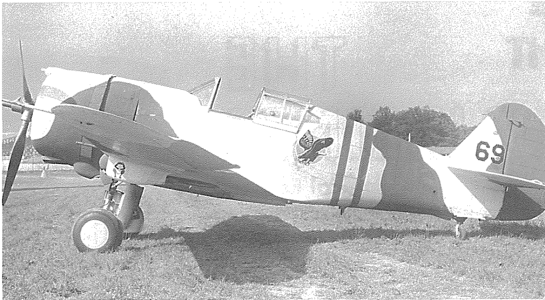
(Left) P-36C camouflaged for 1939 War Games. Note exterior ammunition boxes for wing guns. Ex-P-36E now in USAF Museum has been painted to match this machine. G.S. Williams
