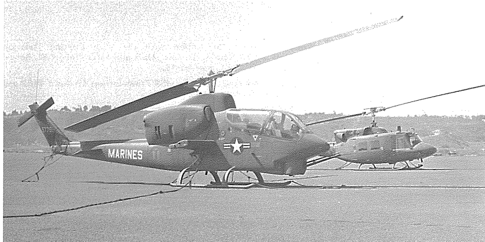
(Below) Marine Corps pilot transition training in AH-1G 815046 at Hunter Army Airfield, Fort Stewart, Georgia. Mid 1969. The large numbers and light-colored areas on the forward fuselage are day-glo orange with the standard yellow tail rotor warning strips around the tail boom. USMC A419214
