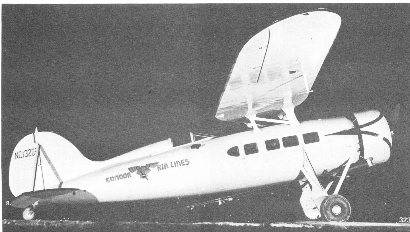
8. Consolidated Fleetster with 575 HP P & W Hornet B1, introduced all-metal monocoque fuselage to US airlines. The Fleetster cruised easily at 160 mph while carrying seven passengers.
