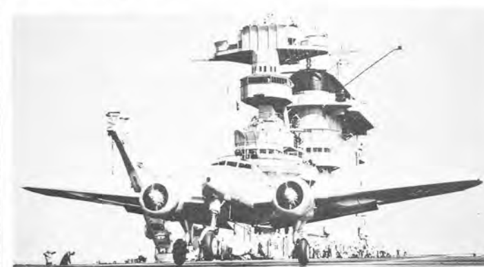
(Above) Rare photo of the XJO-3 taking off from the USS LEXINGTON on August 29, 1939. The initial trials of twin-engine and tricycle gear operations aboard carriers were done with this airplane. (U.S. Navy)
