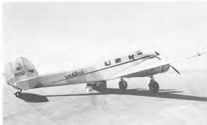
The original Lockheed 12A, c/n 1201. The X for experimental certification prior to approval can be seen on the top of the right wing and on the rudder. At Union Air Terminal, Burbank. (John C. Mitchell)
