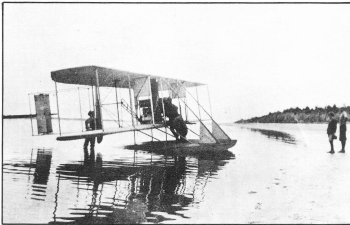
Wright B-1 at North Island, San Diego, 1912. Aircraft mounted on twin pontoons and Wright four-cylinder engine after the aircraft and engine were repaired from March 1st crash. Heath-Paragon propellers installed as shown between April 4 and April 16, 1912. Airplane crashed again with Lt. John Rodgers on 16th. Thereafter twin pontoons were replaced with single Curtiss pontoon. Photo Smithsonian Institution.
