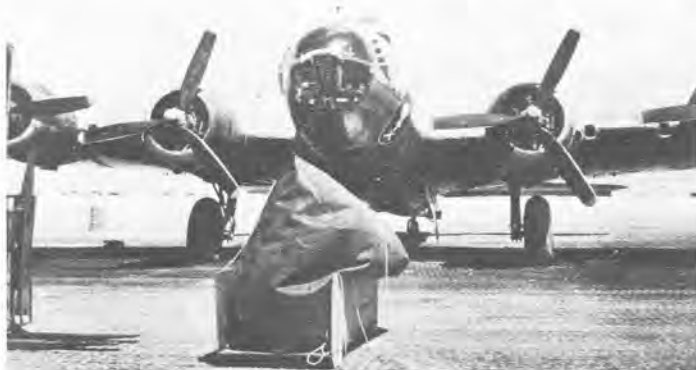
The two photos above are of one of a number of QB-17 drones used in the Operation Crossroads nuclear tests at Bikini Island in July of 1946. The aircraft is pictured here at its Eniwetok Island base prior to its initial sortie through "the Bikini Cloud". The box-like structure mounted atop the B-17 is a "particulate matter sampler". The bag-like device was installed in the bomb bay and used to collect samples of the various radioactive gases found in the atomic cloud. A Bikini drone such as this was later used by Mantz for his famous belly-landing scene. (courtesy Los Alamos Scientific Laboratory)
