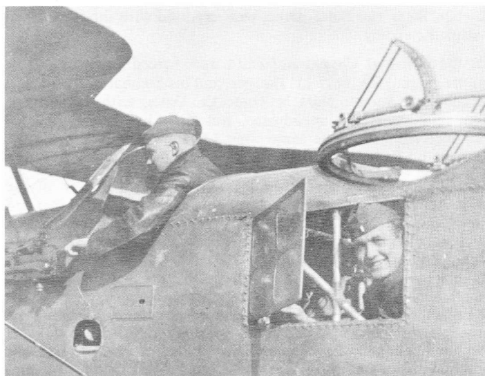
Chapin (in cockpit) and Laird in a training Breguet during early period with French Squadron Br.127. The observers' window and port for fuselage fuel tank are revealed in this unusual closeup view. (Chapin album)
