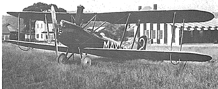
Oriole with C-6 engine at Mayer Field, Bridgeville, Pa., owned by C.P. Mayer, in Summer 1920. It crashed and was rebuilt as racing type similar to one used by C.S. "Casey" Jones. (Kenneth M. Sumney)
