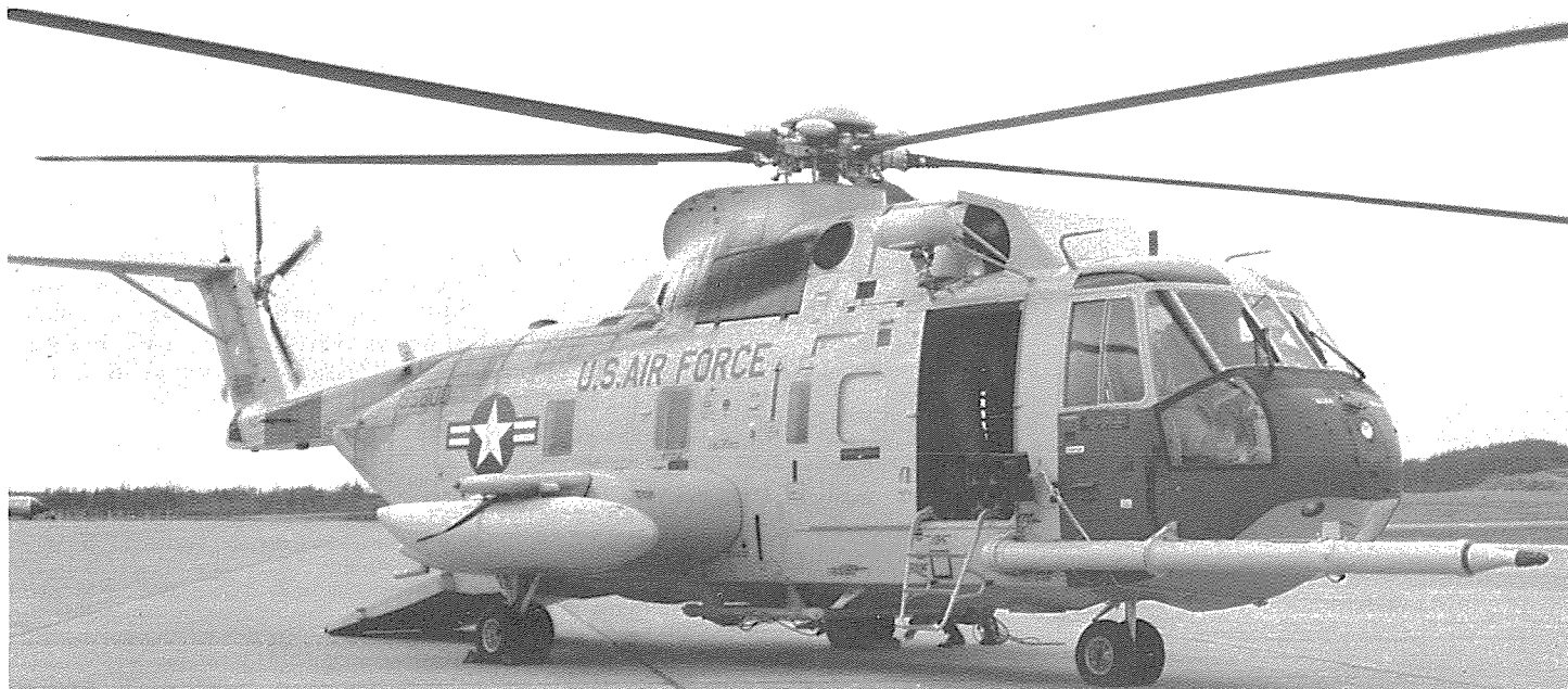
The first HH-3E to arrive in Alaska, 27 April 1970, ferried from Sikorsky plant in 35 hours. 69-5800 of 5040th Helicopter Sqdn. Colors, grey, with red Arctic markings. Equipped for aerial refueling, based at Elmendorf. (Photo — USAF, courtesy of author)
