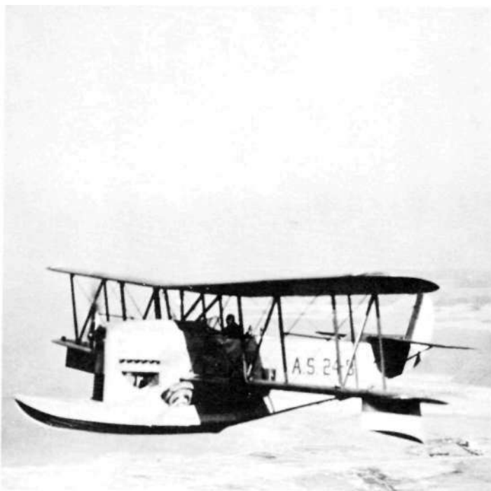
Macready and Doolittle chose the Loening Amphibian for this projected flight across the Pacific. It was a remarkable airplane for its time. Powered by the inverted Liberty engine of 400 hp, it weighed 3,300 pounds empty (with wooden four-blade propeller), and its useful load was 2,200 pounds with 250 gallons of fuel. Shown here is the COA-1, Loening Model 34, c/n 2, over Langley Field in 1924. (Photo - Aviation Magazine, courtesy of Mrs. Sally Macready Liston)
