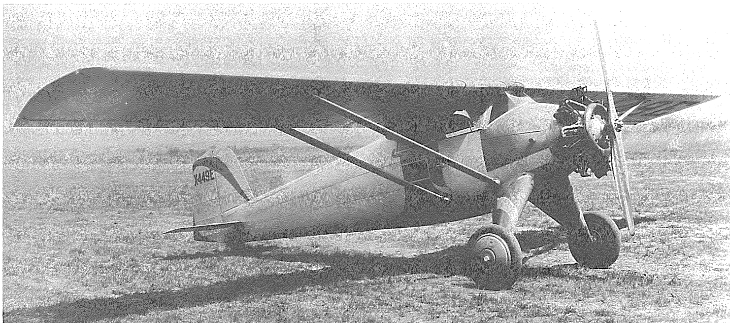
The Fokker H-51, an all-metal monoplane with its original German Siemens engines.
