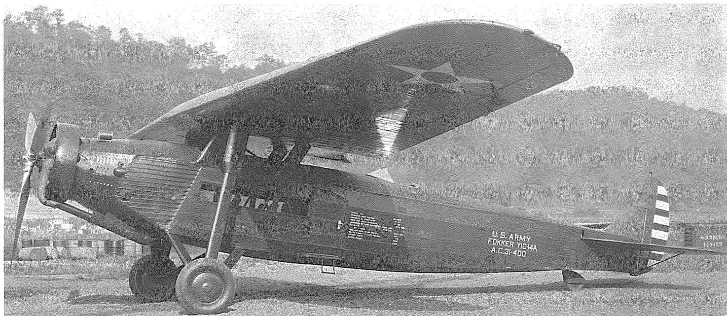
The last Y1C-14 was completed as Y1C-14A with 575 hp R-1820 Cyclone engine and three-bladed propeller.
