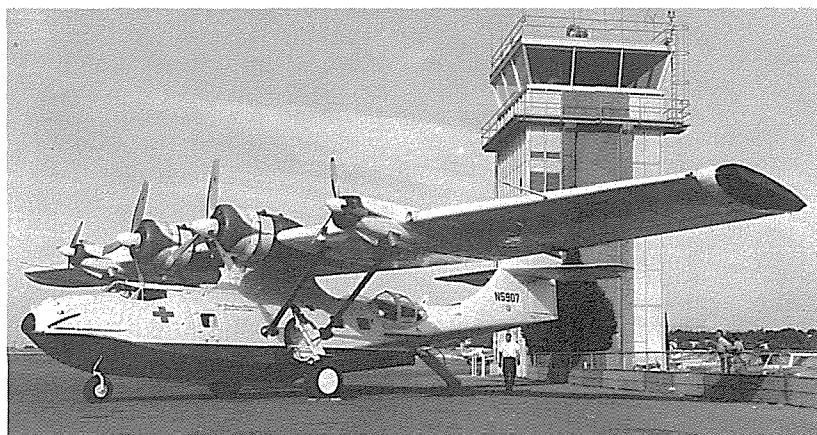
The Bird Innovator, converted from PB5A with addition of Lycoming engines on the outer wing panels, had significantly improved performance to 200 mph cruise speed. Reversible pitch propellers on outer engines aided handling. (Photo—W. T. Larkins)
