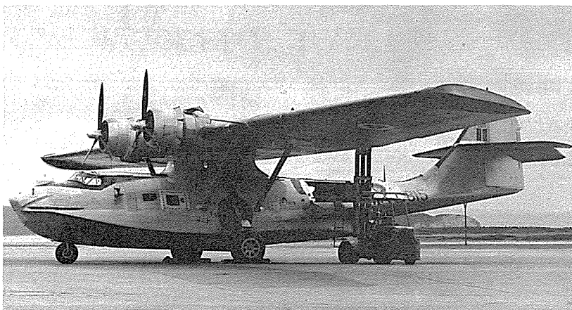
RCAF converted this Canso, No. 9815, to a cargo version, removing the forward turret and blisters, and installing large cargo doors, an astrodome forward of pilot's compartment and minor refinements. Harmon Field, Newf. 1956. (Photo—W. B. Carmody)
