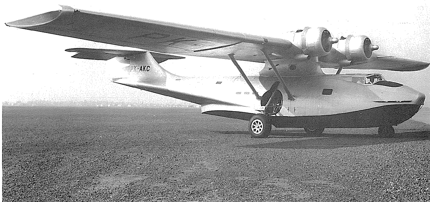
PK-AKC was a typical postwar conversion of PBY-5A, nose turret and blisters removed. Photographed at Oakland, Calif. in Jan. 1947. Pacific Islands Aviation Society reported, in "Balus Na Niu Gini", that PK-AKC crashed at Bangka in 1947. (Photo—W.T. Larkins)
