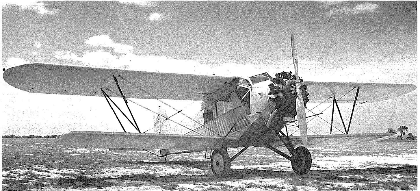
The Cunningham-Hall PT-6 prototype, NX461E, with 300 HP Wright J-6 engine, first flown 3 April 1929. Six-place, all metal structure, fabric covered.
