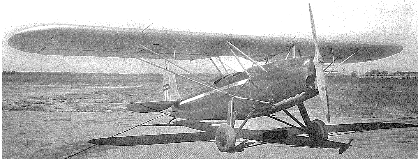
Bureau of Aeronautics procured this Hall high-lift wing example, mounted on a Fairchild 22 fuselage. Shield on rudder states "NACA 60."
