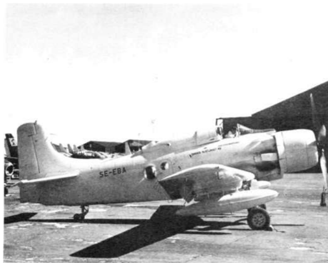
SE-EBA of Svensk Flygtjänst AB, first of the twelve ex-Royal Navy AEW.1s to appear in civil markings. "Guppy" radome entirely discarded, tail hook and many other items of RN operation removed. (Photo - Scottish Av. No. NR/4/1025/962)
