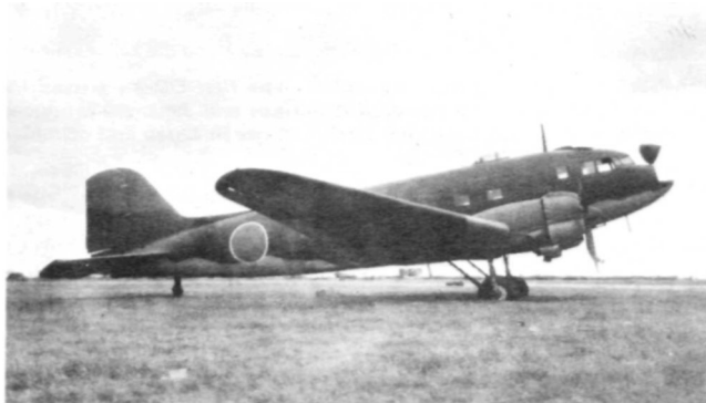
The military DC-3 entered production at Showa in 1940 in a Douglas-type factory facility almost completely imported from America. This is the L2D3 Type O Transport version "Tabby" with top gun position. Fliptop nose stowed cargo. An estimated 490 Tabby's were built between 1940 and war's end. (Photo — Hideya Ando)
