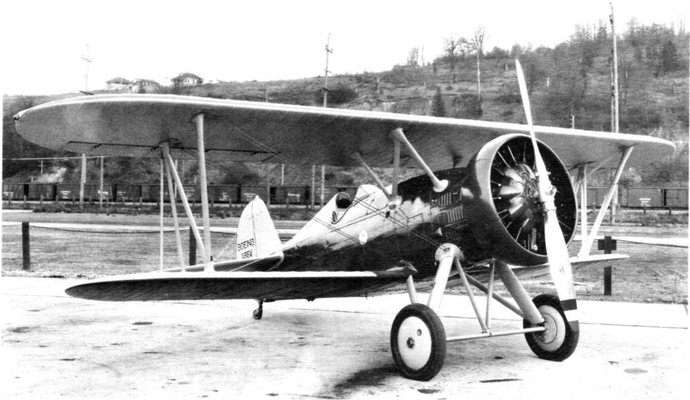
Boeing Model 218, X-66W, c/n 1260, owned by Boeing and used as prototype test airplane for Army and Navy P-12E and F4B-3 series, with Pratt & Whitney engines. Assigned designation XP-925 with
