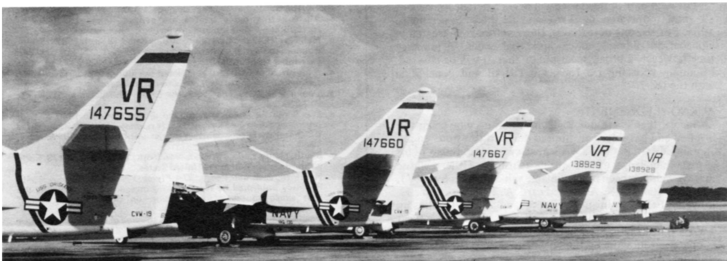
VAQ-130 from U.S.S. ORISKANY at Barber's Point NAS, April 1969. Nearest three, with command stripes, are EKA-3B (Electronic Countermeasures, Tanker, Attack), others are A-3B's. (Photo - Color slide by N.M. Williams)
