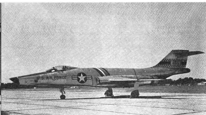
Above—McDonnell YRF-101A-10-MC. "A" and "C" models used Pratt & Whitney J57-P-13 engines, "B" used -55 engine with longer, smooth tailpipe. (Photo—McDonnell D4E-71874). Below left — F-101B-95-MC. J.O.683 on fin is inhouse job number. (Photo—Dean S. Engelhardt). Right—RF-101A-30-MC of B/Gen. Stephen B. Mack, C.O. of 363rd TRW, Shaw AFB, S.C. (Photo USAF courtesy of author).
