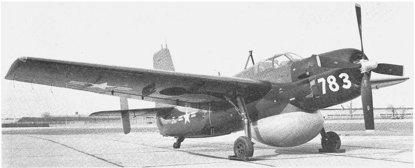
No mistake that this is the search half of the submarine hunter-killer team, the AF-2W Guardian. The engine was the R-2800-48W of 2400 hp. (Photo — GAEC G-38580)
