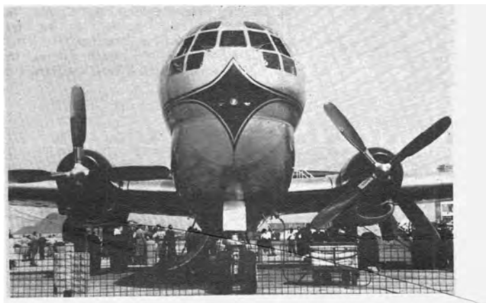
Figure-8 fuselage and cockpit window area are apparent here on AOA's FLAGSHIP EUROPE. AOA used Curtiss Electric Propellers, other airlines used Hamilton Standards. (Photo F. Dominie)
