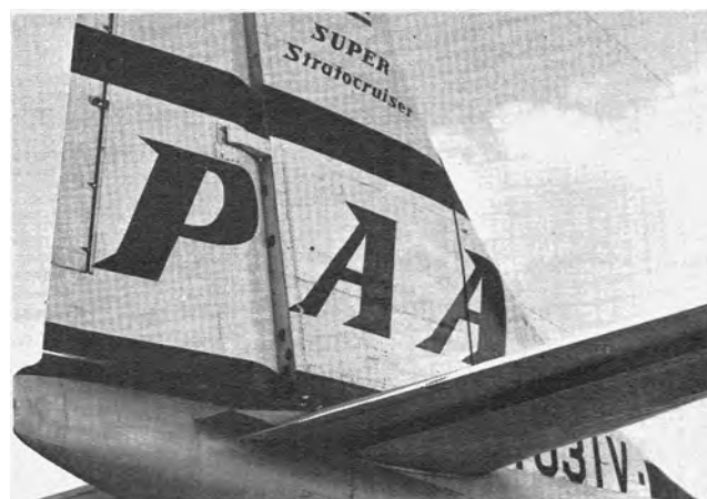
Distinctive fin marking applied to those with additional fuel tanks for non-stop flight from New York to London or Paris, shown here on N1031V, one of ten so modified by PAA. (Photo-PAA)
