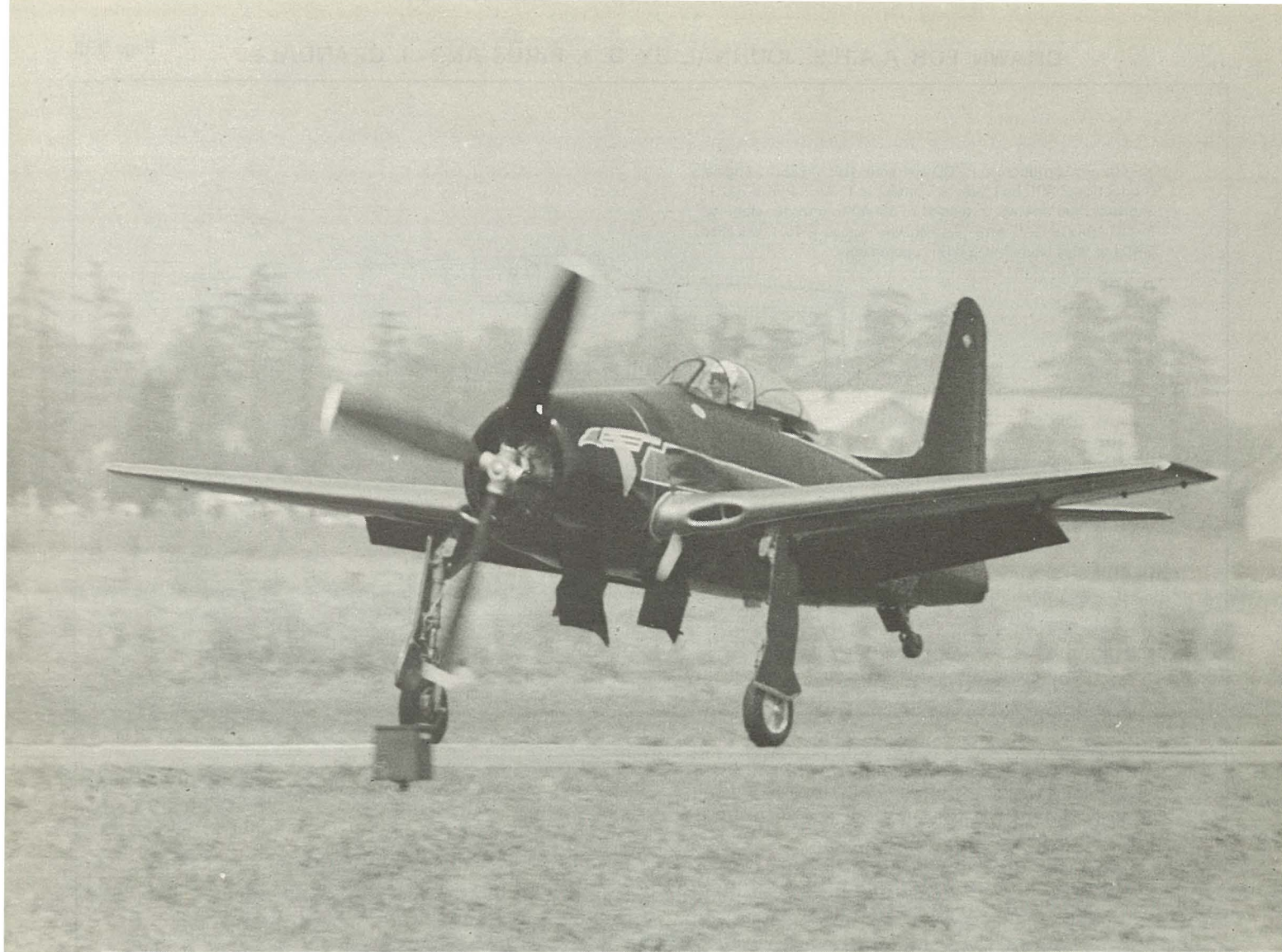
Grumman F8F-2, BuNo 121787, now N148E, at Bracket Airport, near Pomona, California, late 1968. Owned by John Church of Carmel. Colors, black, gold trim, white pin stripe. Raced at Reno 1966 & 1967, carried Race Number 11. Was red with white trim in 1966. As "stock" Bearcat, lightened by removal of armor, it placed Third in Unlimited Class in 1967 at average speed of 331 mph. (Photo — Tim Piedimonte, 67-5-22-28)
