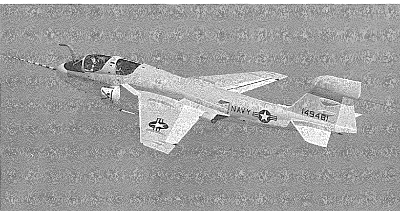
Latest Intruder development is EA-6B four-place electronic warfare aircraft, undergoing extensive flight testing. The number one airplane was built from Grumman shop No. 15, with a 40-inch section spliced into fuselage for rear seat locations. Large bump on rudder
