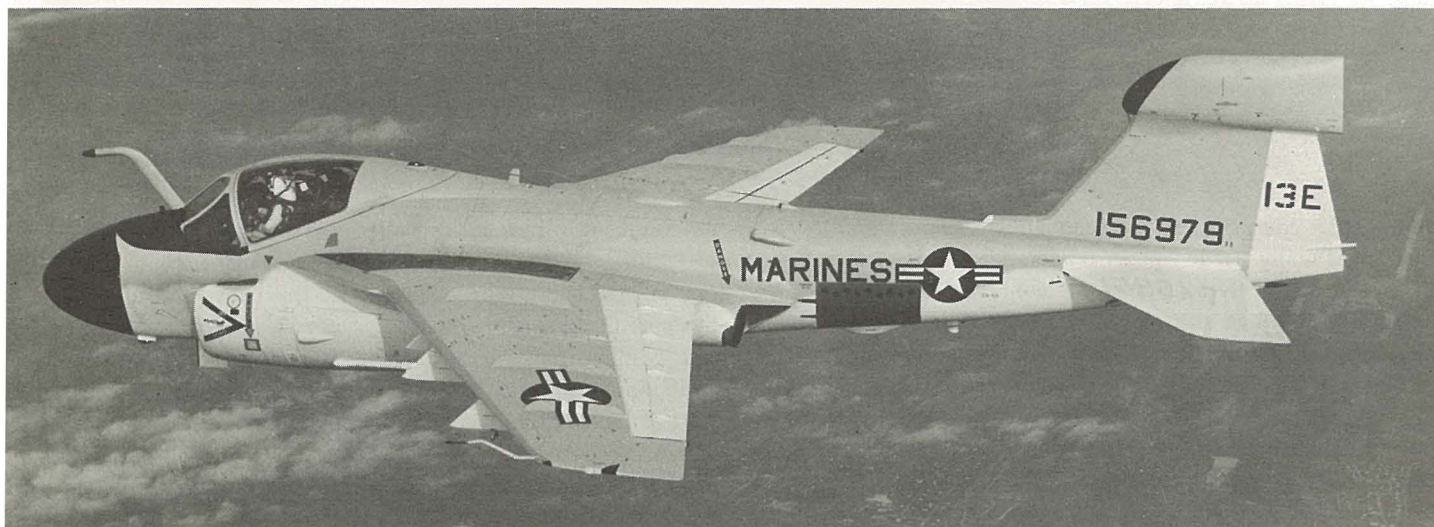
The first of the USMC/Grumman EA-6A airplanes. Black radome and fuselage speed brakes retained, airspeed boom remains on port wing as in early A-6A, and no wing tip brakes. (Photo-Grumman 681104)
