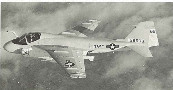
Although shown elsewhere, this photo is included to indicate, for comparison, the latest configuration of the A-6A, with white radome, airspeed boom located on vertical fin again, fuselage speed brakes deleted, wing-tip brakes included. (Photo - Grumman No. 681044)
