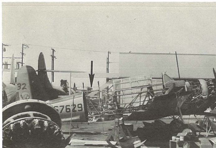
Val/ex-BT-13. Arrow points to 26" extension in fuselage.
