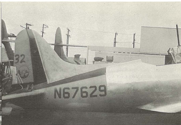
Val after re-skinning, with fibreglass fin installed.
