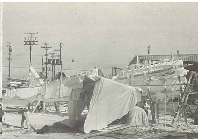
A plastered P-40. Same P-40E in a plaster cast. The cast was later used for manufacture of fiberglass P-40 fuselages for movie props in filming of attack on Pearl Harbor. (Photo — Mauno Salo)
