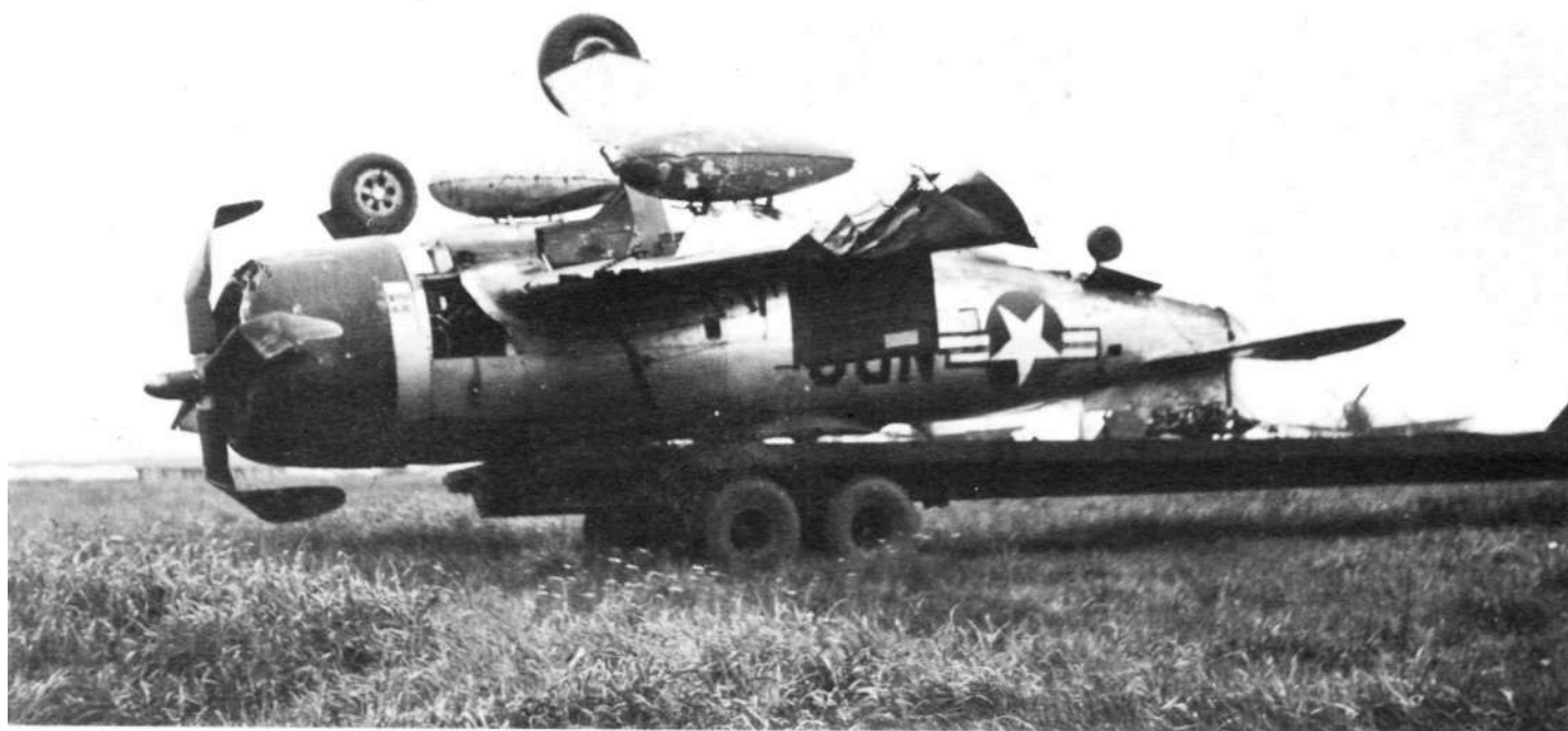
ND-8 of the 527th, dropped a wheel off the runway on landing and flipped over. Pilot injured.
