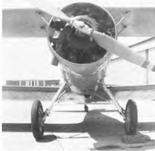
Study of N3N-3 landing gear, simplified from earlier N3N-1. Track is 6 feet, wheel size 30x5. Note outward camber of the tires and 9-foot Hamilton Standard prop. (Photo: Author).
