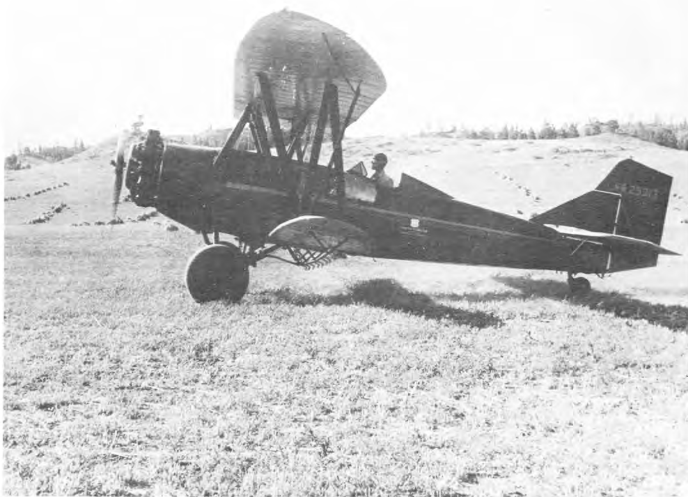
White New Standard NR 25313 (C/N 167W) with spray boom installed. This aircraft was the last delivered by White Aircraft Corporation and the last New Standard built. This was the only one of the New Standards built for the USDA which was equipped with a Hamilton Standard two-position propeller, the others being equipped with ground adjustable propellers. (USDA photo Bn30171)
