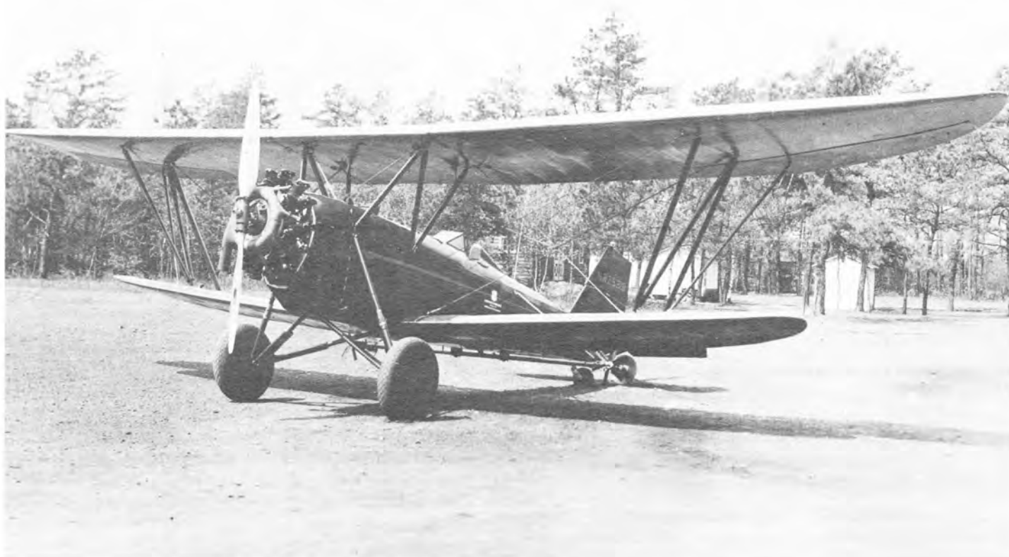
White New Standard NR 25319 (C/N 166W) with spinning disc atomizer for handling slurries. This aircraft was the last of the New Standards belonging to the Bureau of Entomology and Plant Quarantine to be operational. (USDA photo Bn30170)
