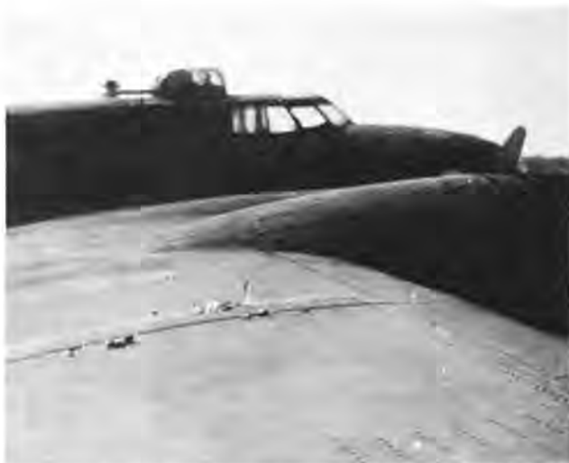
Japanese 20 MM shell damage to B-17 wing in air combat, March 1942, 19th Bomb Group. (Photo - Logan)
