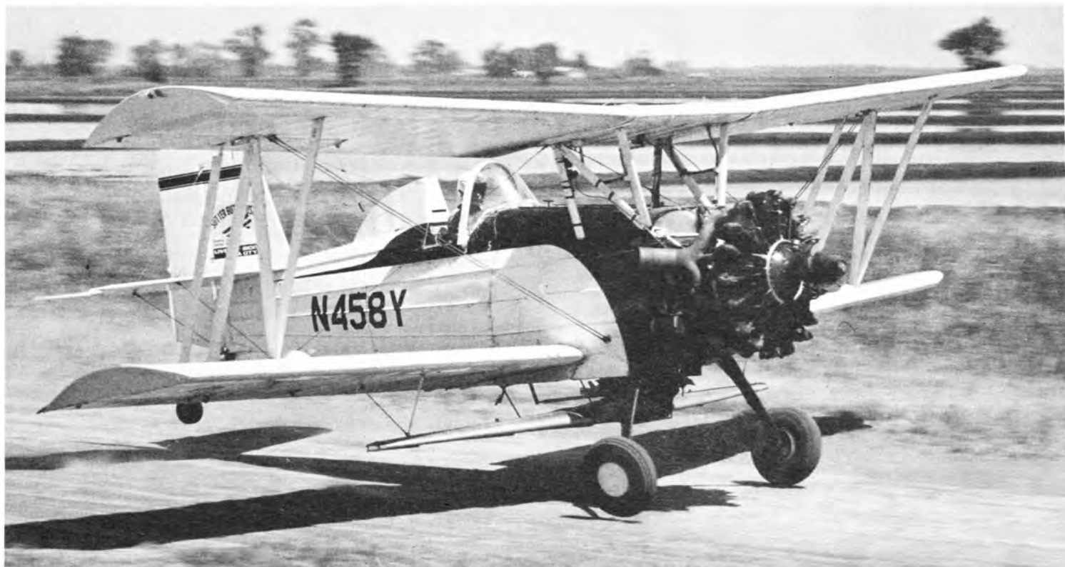
A highly modified Grumman G-164 Ag Cat - typical of present California operations. The 600 hp P&W R-1340, windshield and Swathmaster are all modifications. Sutter-Butte Dusters operates a fleet of these in the fertile rice fields of Northern California. Photo in April 1966 near Sutter, Calif., by W. T. Larkins.
