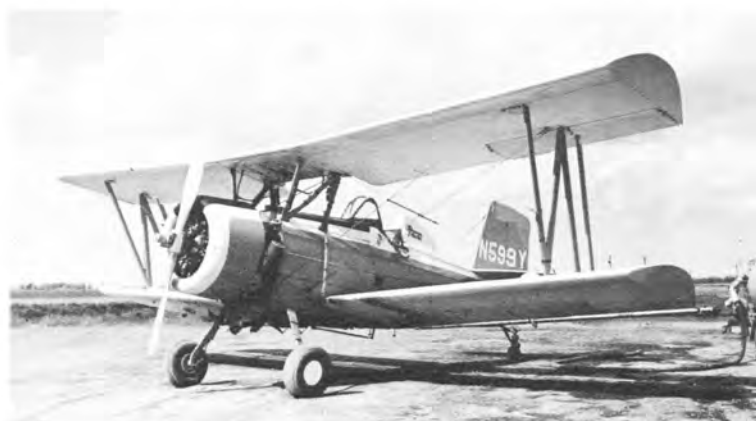
Many Ag Cats are flying with the P&W R-985, 450 h.p. engine, from the BT-13. This one, of Thayer Brothers also has a BT-13 cowl and windshield. 1966 (Larkins)
