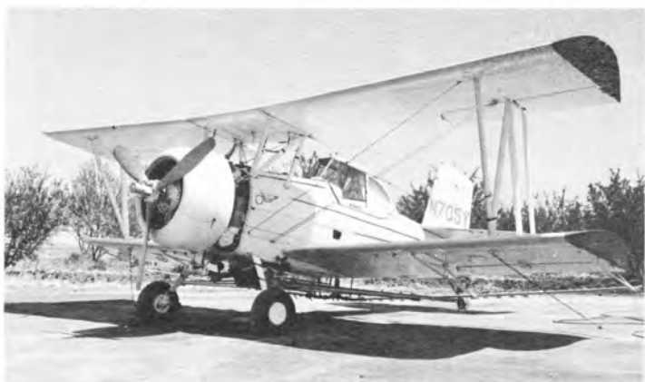
A rare one-only with AT-6 engine and cowl and three-bladed prop from DeHavilland "Otter," extended wing booms and extra lights for night flying. (Larkins)
