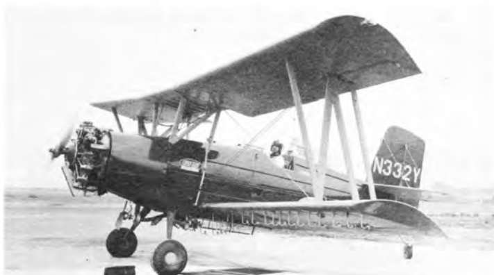
The more normal G-164 with Jacobs R-755A of 300 h.p. and factory installed wing nozzles. McLoughlin Dusters, Oxnard, Calif. November 1965 (Larkins)
