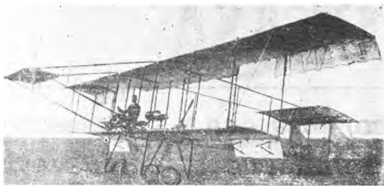
The Farman type Noni, with a 50 hp Gnome engine.
