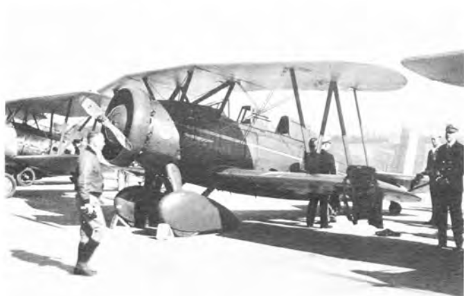
Curtiss XO2C-1, USN A-8845, in 1931 as dark blue Flagplane for admiral's use. Was designated XF8C-7 before and after this period. (Photo - U.S. Navy via F. Dickey, Jr.)
