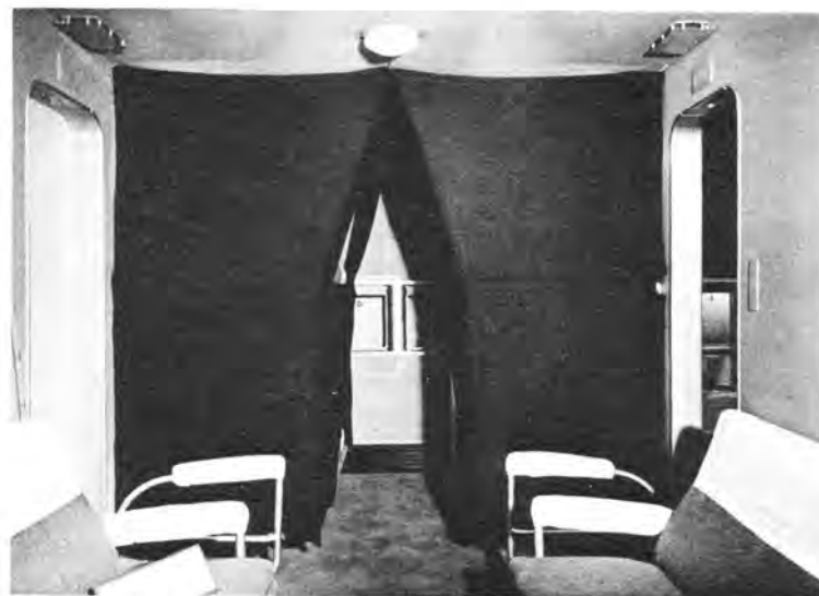
A standard-passenger stateroom, as found aboard a Boeing Clipper, shown in day and night arrangement. Each standard compartment held 10 passengers by day, six by night. (Author photo)
