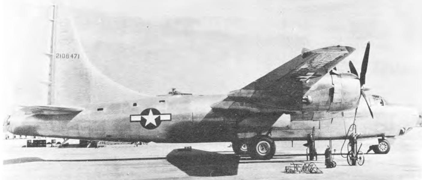
Ultimate revision, bringing B-32 its most distinctive feature, raised fin height to 19-1/2 feet. (Convair)
