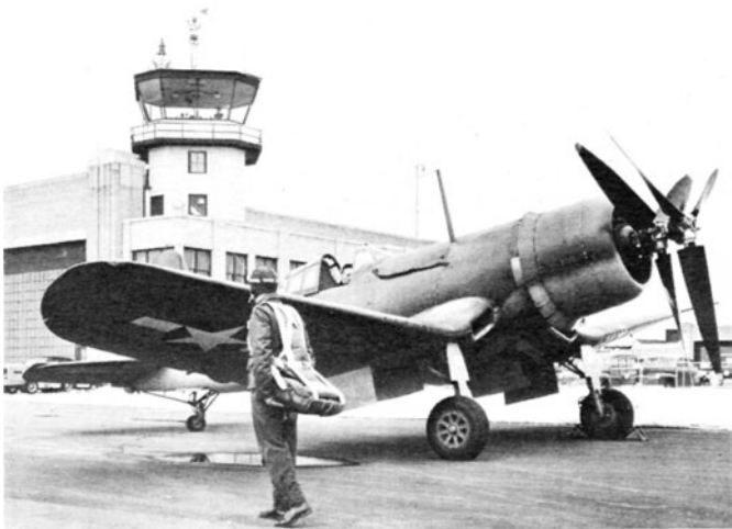
Experimental 1944 installation of contra-rotating prop on F4U-1 by Pratt & Whitney Aircraft. Engine used was P & W R-2800-55. (P & W Photo)
