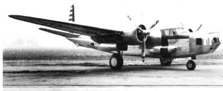
the alternate nose configuration, the "B" nose, was installed, machine-gun packages added. In DB-7 the guns were moved inside the fuselage. (Photo-Douglas)
