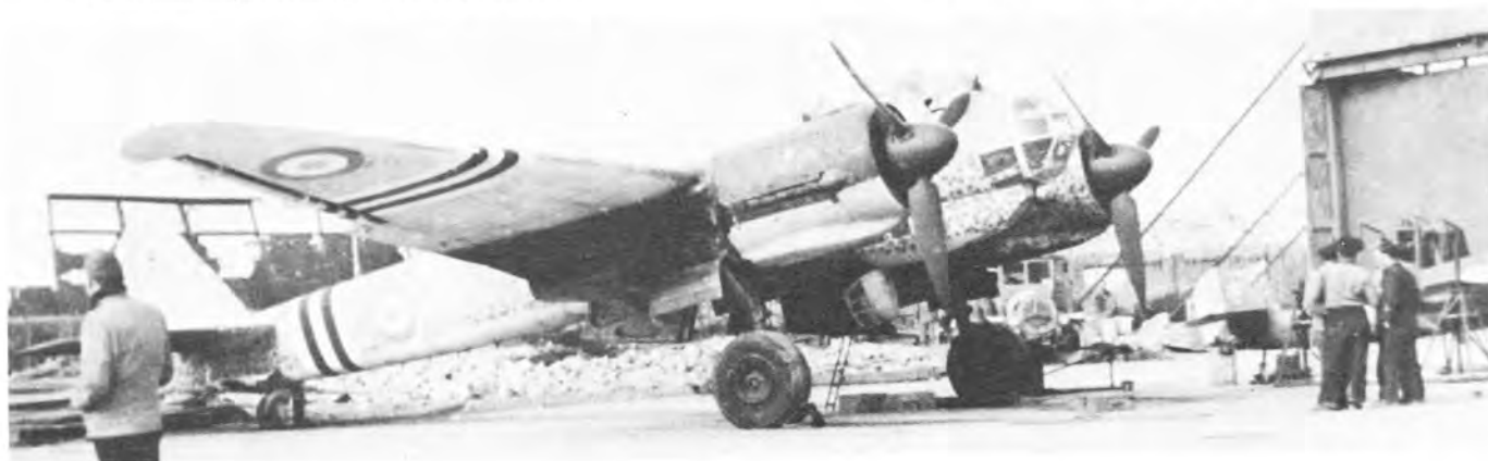
Ju 88A No 5 after replacement of damaged right engine cowl by spare of different color from A.A.B. production line.
