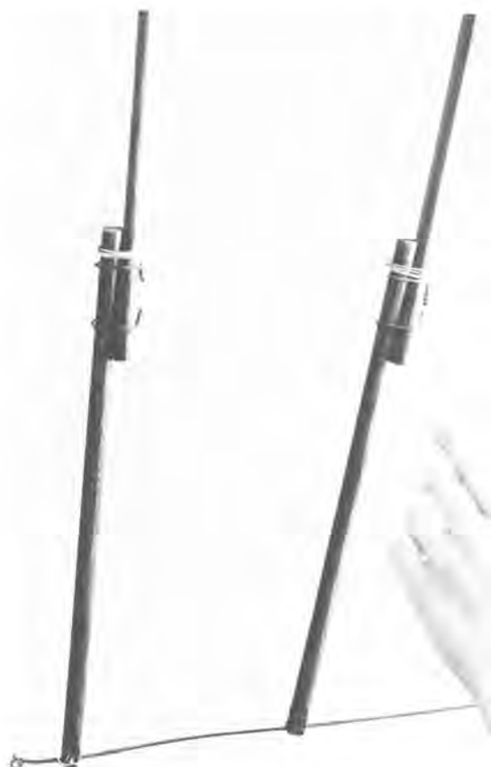
Trailing edge of the original wing of the Evergreen glider, showing last day splice that resulted in sustained flight.
