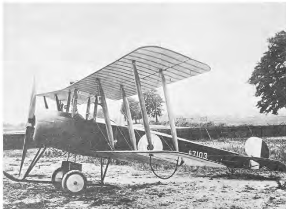
The airplane that made Avro a leading manufacturer of British aircraft, the Model 504. This is a 504K manufactured by Hewlett & Blondeau during the First World War, one of 17 firms that turned out 504s besides A. V. Roe and Co. (Courtesy Hawker Siddeley Aviation, Ltd.)
