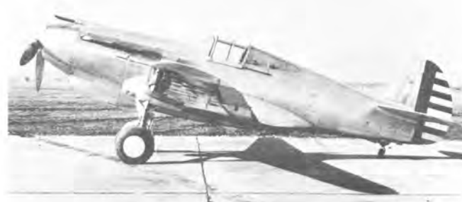
The XP-40 after modification placing the engine coolant radiator under the nose and adding new exhaust outlets. (Author)
