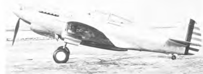
After second modification the XP-40 took this final form with landing gear fairing plates removed and cleaned up nose. (Author)
