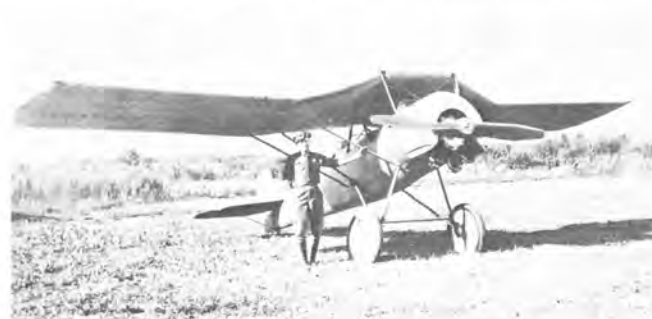
MB-10 two seat trainer, conceived at same time as MB-9 to complement it. Both were flown only as prototypes and exhibited vestiges of the "Alula" principle. (Matt Coll.)
