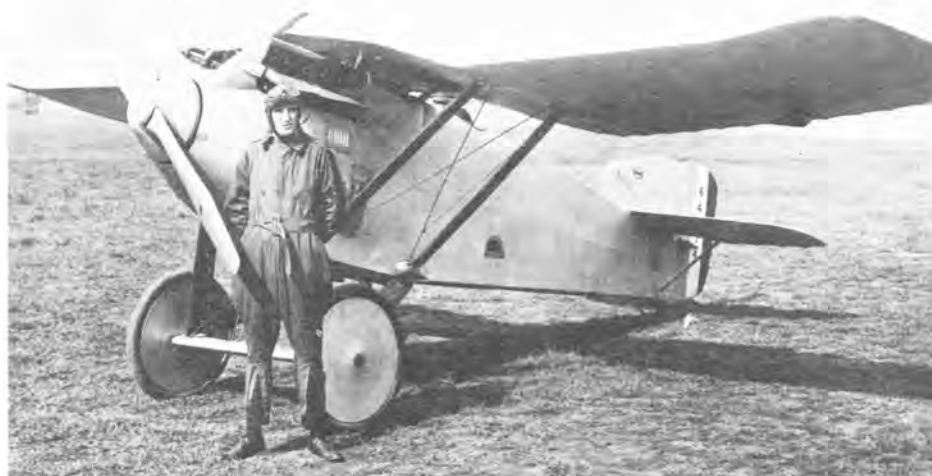
Capt Francis P. Mulcahy, a Marine pilot, flew the second MB-7 in the 1922 Pulitzer but did not finish. This aircraft was equipped with the H-3 "Super Hunter", a larger powerplant than used on its predecessor. (National Archives 80-HA-74-1)
