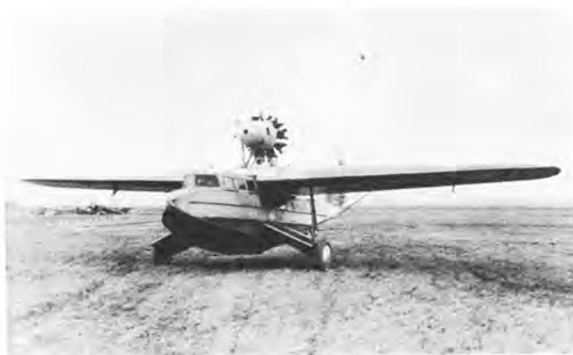
The first, and only, F-11 in its original configuration with short-span Super Universal wing, P&W Wasp engine and moveable sponsons that doubled as landing gear legs. (Fokker Photo)
