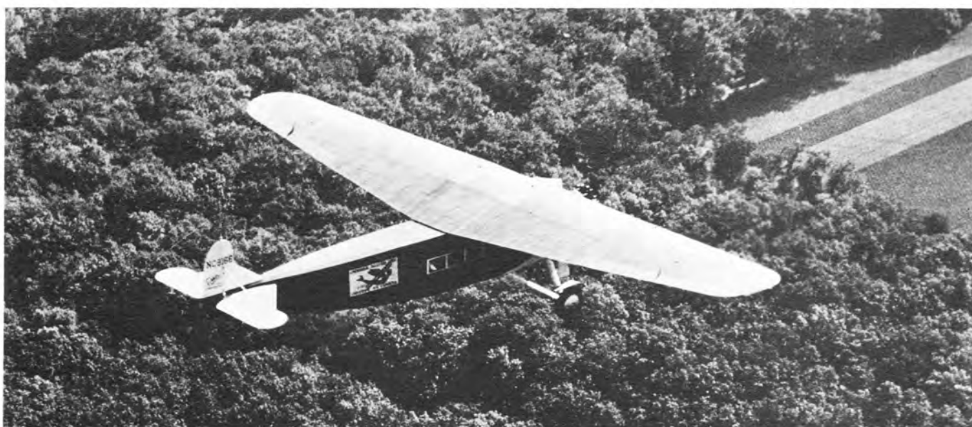
Universal Airlines' F-10A, NC-9166, C/N 1037, showing the straight taper of the F-10A wing from the fuselage to the tip of the wing. The earlier F-10 had parallel leading and trailing edges out to the nacelles. (Universal Airlines)
