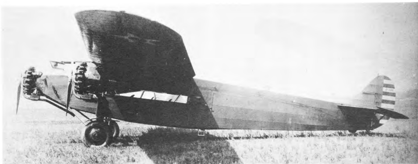
The last Army C-2A, 28-126, was sent to Wright Field for engine change and was redesignated C-7. While under test as XC-7 it carried the Wright Field test number, XP-545. (Wright Field)
