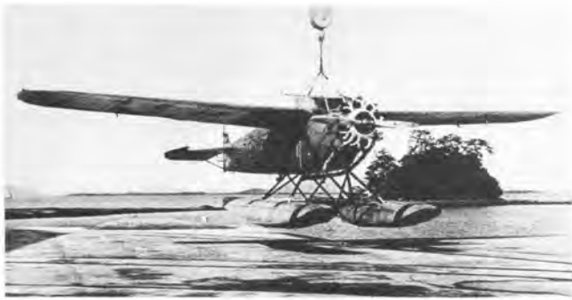
American-built Super Universal seaplane, C/N 857, exported to Japan and fitted there with a Bristol Jupiter engine. Registration is J-BBPO. (Japanese Photo from Shiro Ogiwara)
