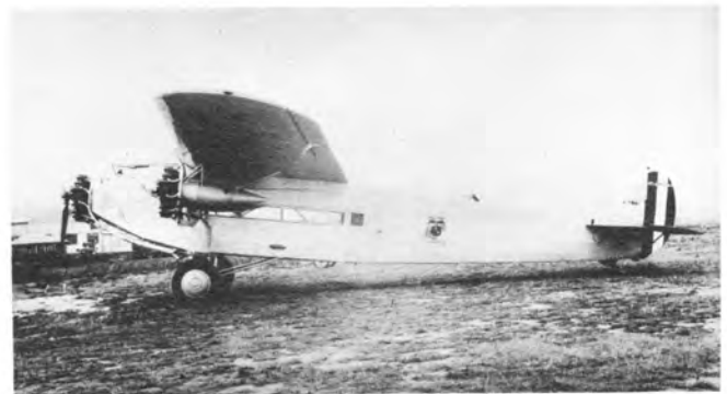
Marine Corps TA-1 was identical to Army short-wing C-2s. This one was fitted with a three-blade propeller on the center engine. (American Fokker Photo via E. M. Sommerich Coll.)
