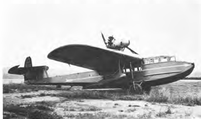
Fokker F-11AHB, C/N 904, registration NC-127M, powered with P&W Hornet engine of 575 hp. This was a deluxe model for famed boat racer and builder Gar Wood. (Courtesy Ben Haines)
