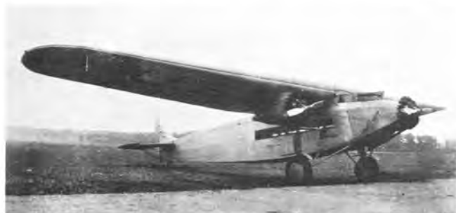
Top, Marine Corps' third TA-2, A-8018, which duplicated the Army C-2A's. This one is on its way to Nicaragua with a replacement wing for another airplane tied under its fuselage. Middle, short-wing Marine TA-1/RA-1 converted to RA-3 by change from 220 hp Wright J-5 engines to 300 hp Wright J-6s. This particular plane, A-7561, has reverted to two-blade nose propeller. Bottom, Marine TA-2/RA-2 also converted to RA-3 by change to J-6 engines with no distinction made for length of wing. Modification to this aircraft, A-8018, includes a large fillet between the tops of the nacelles and the underside of the wing. (U.S. Navy, U.S. Navy and Fred Bamberger)
