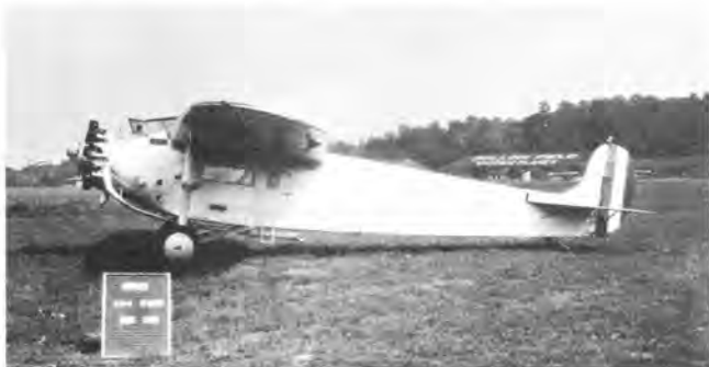
The XJA-1 Super Universal tested by the U.S. Navy in October 1928. Identification board is typical of Anacostia photos. Fokker made several markings errors, leaving off the wing stars and the name "U. S. NAVY" on fuselage. (USN AN-6751)
