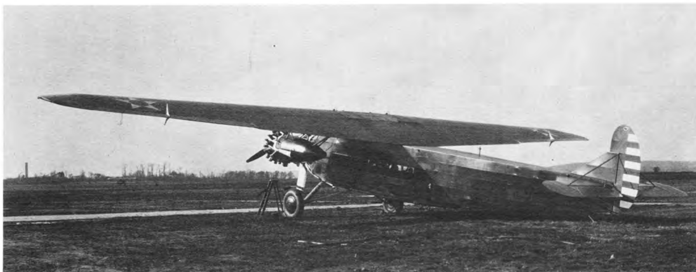
The Army bought one F-10A, with straight lower longerons, and designated it C-5, serial 29-405. (USAAC via Stephen J. Hudek)
