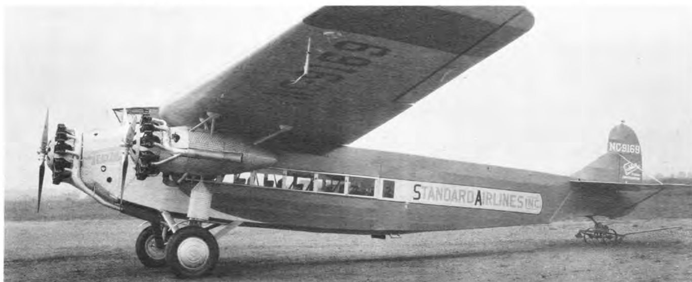
Early F-10A's had straight lower longerons as F-10s, later had reflexed longerons to accomodate steerable tail wheels. NC-9169, C/N 1038, retains a tail skid, shown on ground handling dolly, but has modified longerons. (Fokker Photo 1202)
