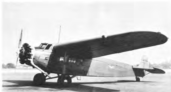
Production Super Universal, featuring a fully cantilever wing, at Alhambra, California, May 7, 1939. (Boardman C. Reed)
