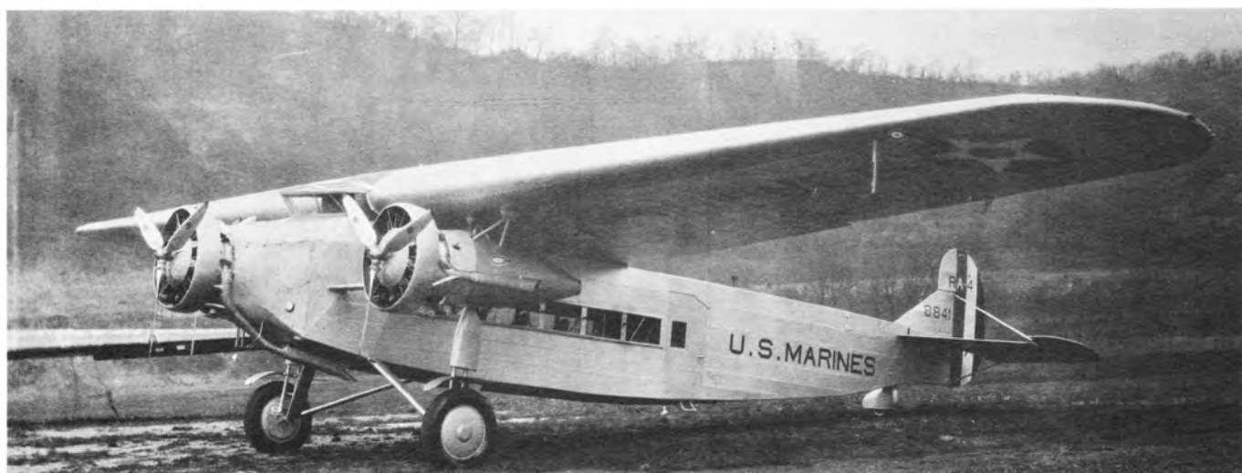
Standard F-10A delivered to Marine Corps as RA-4 in January 1931 with faired steerable tail wheel. (Fokker Glendale 454)
