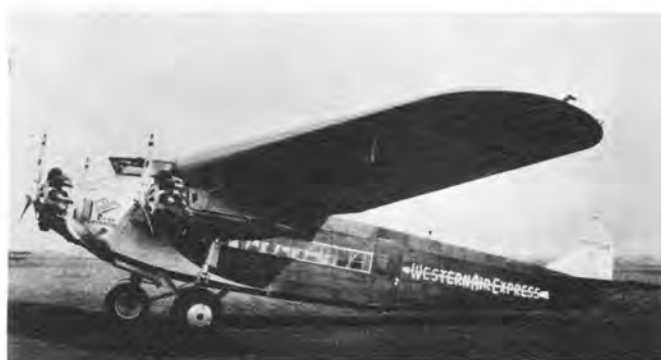
The 1930 Fokker catalog carried a photo (left) of the nonexistent F-9, which was a heavily retouched copy of an original photo of the sixth F-10, NC-8048 (right), changing Wasp engines to J-6s and eliminating Western Air Express markings.
