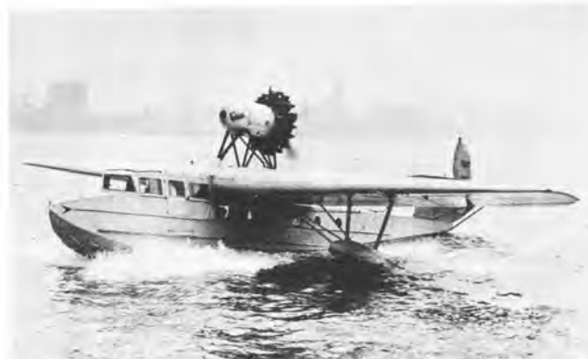
The Fokker F-11, registered 7887, converted to a straight flying boat with wing floats, longer F-14 type wing of 550 sq ft and Wright Cyclone engine of 550 hp. (Stephen J. Hudek)
