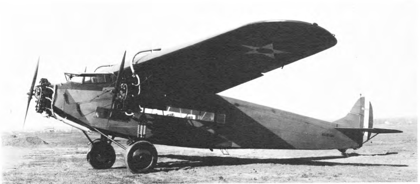
Third U.S. Army C-2, 26-204, delivered in April 1927, in overall olive drab finish with the old Army tail stripes. The Army had two C-2s with the "short" 63-foot wing of the original F-VIIA trimotor. (American Fokker 519)
