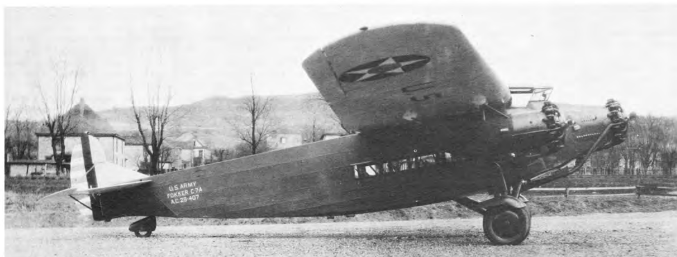
The first C-7A, March 11, 1930, with original F-10 type tail. Fokker again "goofed" with the U.S. national marking, having the red centers of the stars touching the inner edges of the blue. (Fokker Glendale Plant 102)
