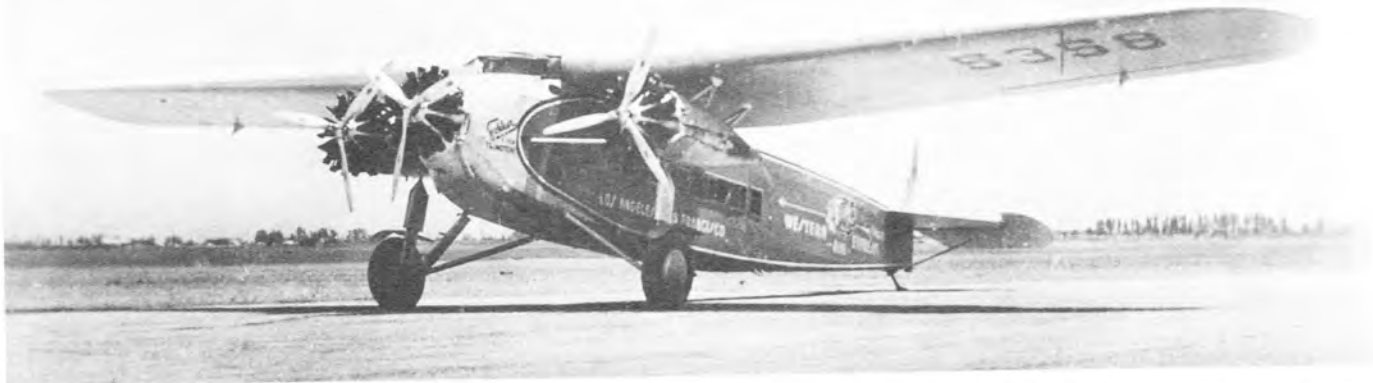
The third Fokker F-10, built for Western Air Express. C/N 1002, registration 5358. F-10s operated under Category 2 Approval certificates and went into service without the letters NC in front of their registrations. (Western Air Lines)
