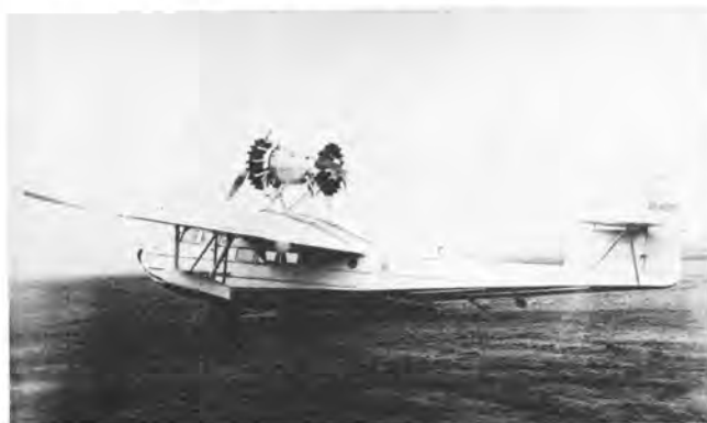
F-11A, C/N 902, registration X-148H, temporarily fitted with an F-32 type nacelle, carrying two Hornet engines. Photographed at Teterboro on March 5, 1930. (Fokker Photo 1493)
