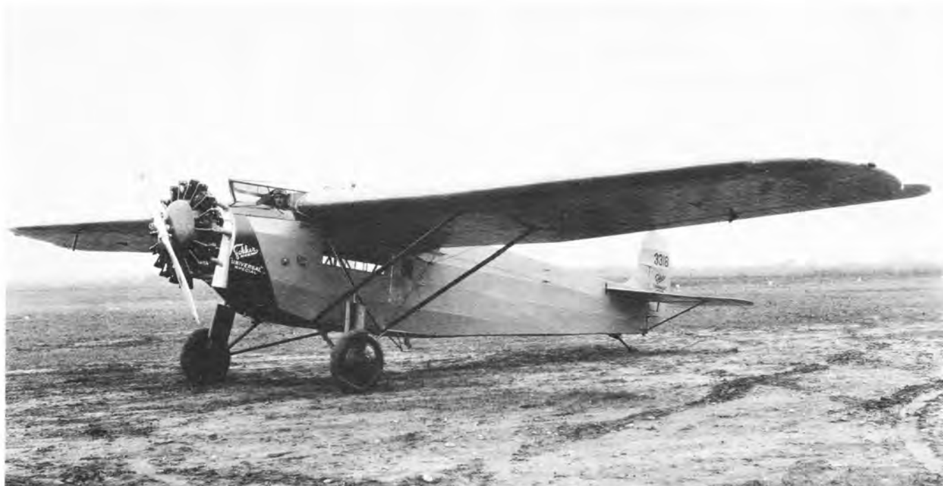
The prototype Super Universal. This name became official for this one-only airplane, appearing in company publicity and FAA records, even though "UNIVERSAL SPECIAL" was painted on its rudder. "C/N 800" is above lower longeron. (Fokker Photo 686)
