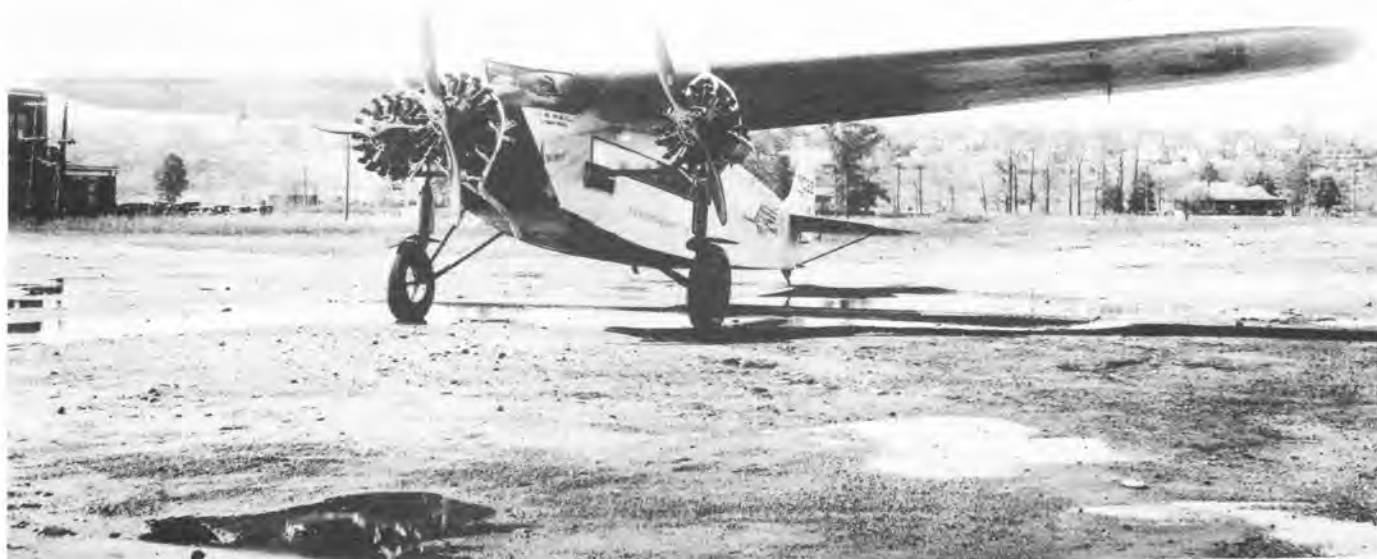
Pan American Airways' C-2, NC-53, which was purchased as an F-VII. Designation "TRIMOTOR C-2" can be read on the nose along with the original name "KEY WEST". The name was later changed to "GENERAL MACHADO" for the Cuban "Strong Man" of the times. The engines were Wright J-5s. (American Fokker Photo from files of Western Flying Magazine, 1950)
