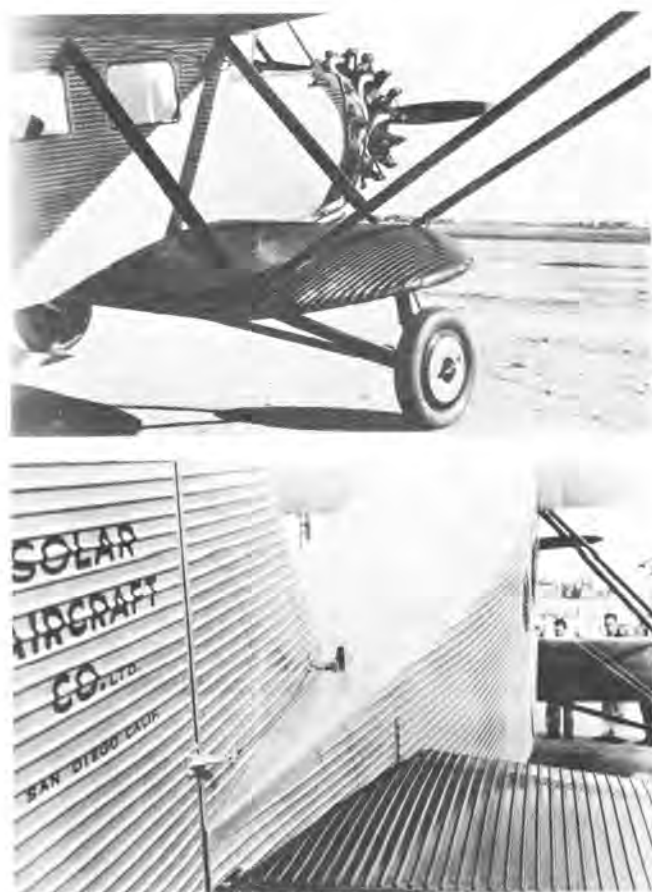
Sesquiplane and tail configuration of the MS-1, (Solar)
