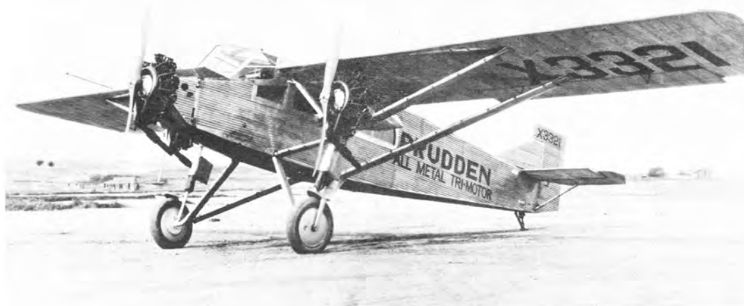
Prudden XM-1 with three Ryan-Siemens engines as seen in 1927 on a field near San Diego. (Peter M. Bowers)
