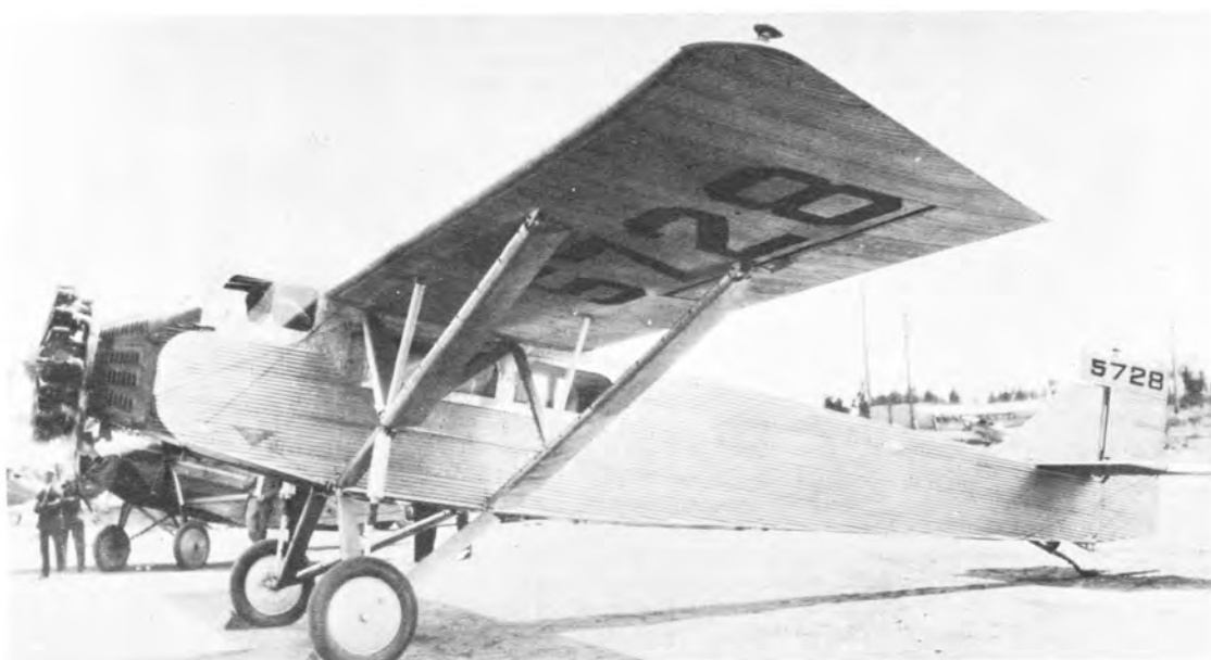
Modified to single engine configuration with Pratt & Whitney Wasp, the TM-1 became the SE-1. (Peter M. Bowers)
