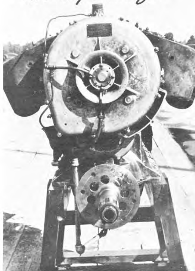
General Electric turbo-supercharger installed on 12-cylinder Liberty engine. (U. S. Air Force)
