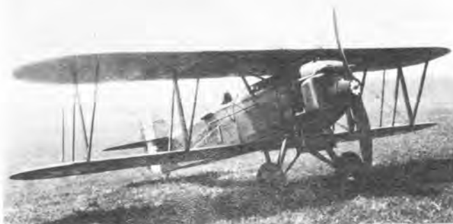
Curtiss PW-8, 24-202, was first turbo-supercharged Curtiss pursuit. Tested at McCook Field, 1925-26. (M. Copp)
