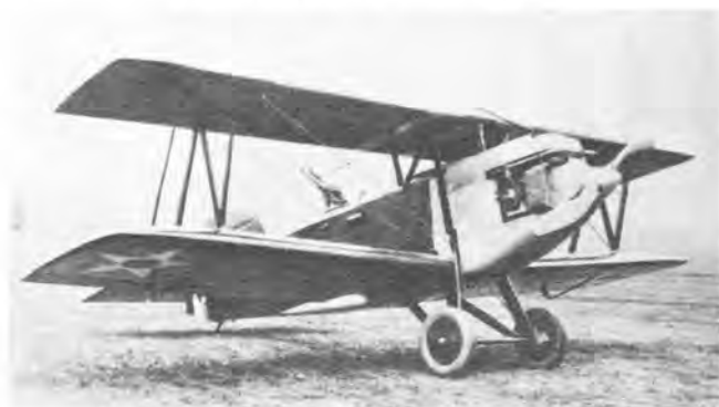
TP-1 with side mounted, Type F turbo-supercharger while being tested at McCook Field. (Author)
