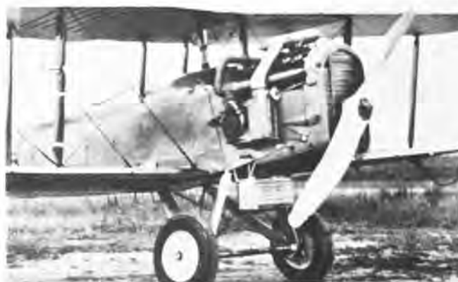
NACA aircraft Number 25 with turbo-supercharger. This DH-4 was also flown with other types of superchargers. (NACA)
