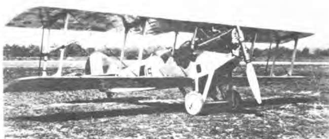
LePere LUSAC-11, 40015, with very early form of turbo and a variable pitch propeller. (Marty Copp Coll.)
