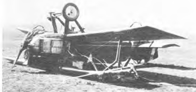
Engineering Division TP-1 with front mounted turbo, after crash at McCook Field. (R. Cavanagh Coll.)
