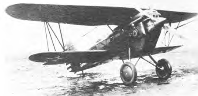
Curtiss XP-5, converted from P-1, at McCook Field with F-2 turbo-supercharger unit installed. (USAF)
