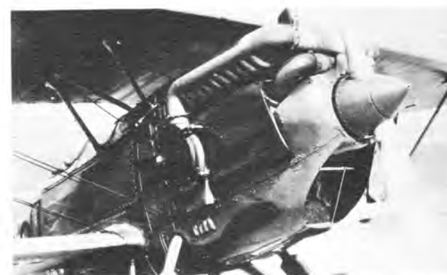
Curtiss XP-6D, 29-260, turbo installation. This was only P-6D to have 2-bladed propeller. (R. Cavanagh)
