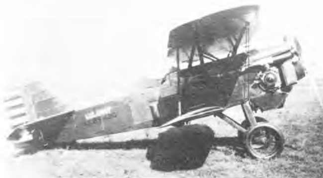
The Curtiss P-2 was tested with turbo-supercharger at McCook Field as XP-431 in 1928-29. (M. Copp)
