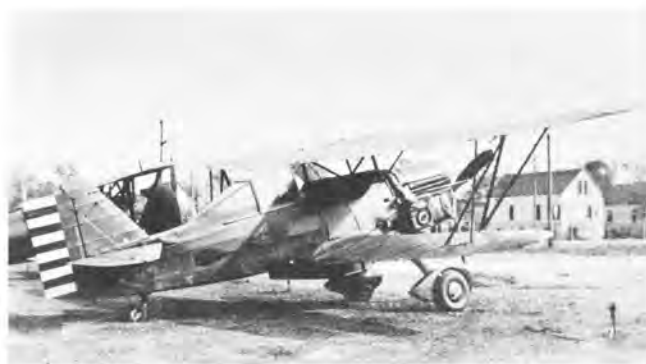
Wright Field based Curtiss XP-6F, 29-374, was modified XP-6E with F-2 turbo-supercharger. (E. C. Haney)
